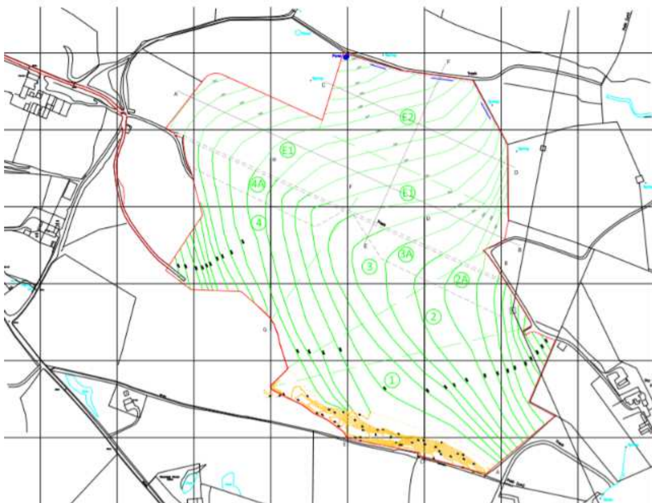
Restoration contours and phasing
